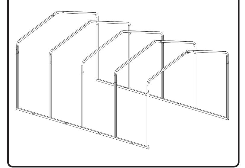
NOTE: The 12'W x 20'L x7'H is a base building. Buildings longer than 15' will receive 2 additional boxes for each 4.5', one frame box with 1 middle rib and one panel box with 7 middle panels. These frames and panels are inserted in the middle section of the base building. **Extension Module Parts Part Name** Qty G 803562 Н 803468 804859 2 K 803466 2 L 803467 2 11061
