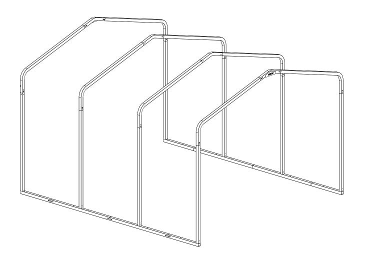
NOTE: The 10'W x 15'L x7'H is a base building. Buildings longer than 15' will receive 2 additional boxes for each 4.5', one frame box with 1 middle rib and one panel box with 7 middle panels. These frames and panels are inserted in the middle section of the base building. **Extension Module Parts** Qty **Part Name** G 803562 Н 803468 804859 2 803466 2 K L 805682 2 11061 6 M 11066
