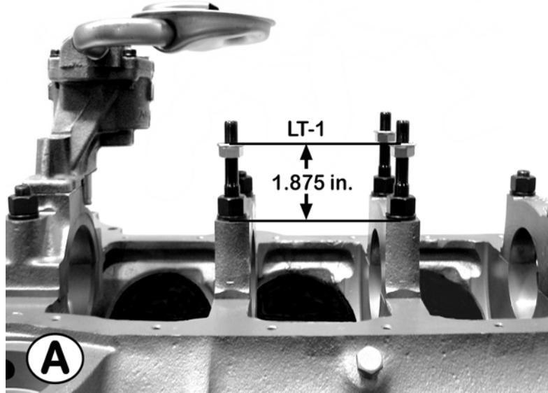
1. Check for a minimum of .020 in. clearance between the nut on the rear main cap and the oil pump housing.
