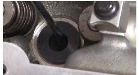
PATTERNED SIDE DOWN on dry spot face on the head
