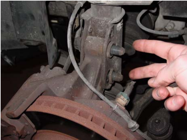
9. Remove the two nuts at the bottom of the strut. ↑
