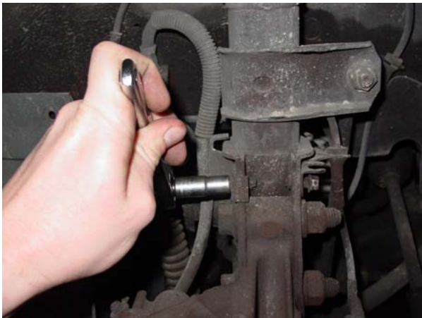
3. Unbolt the 2 side brackets from the strut. ↑ (These brackets hold the brake lines and other cables)
