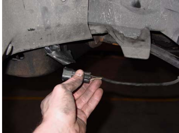
8. Unplug the strut damper solenoid. ↑
