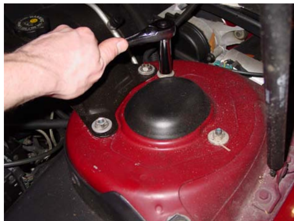
13. Remove 3 nuts attaching top of strut assembly to body. ↑
