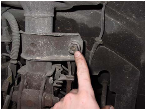
5. Remove nut from stabilizer link ↑
