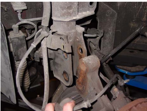
11. Knuckle will fall away from strut. ↑
