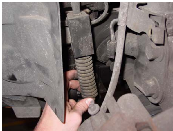
4. Remove the position sensor from upper and lower ball studs. ↑
