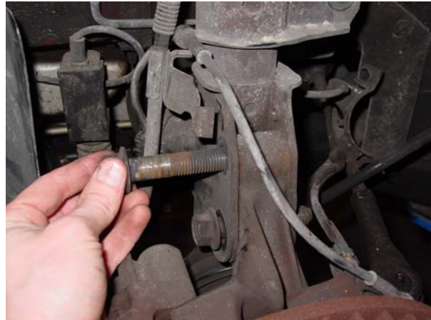
10. Remove the two strut-to-knuckle bolts. ↑
