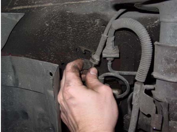
7. Remove strut damper solenoid cable from mounting brackets. ↑
