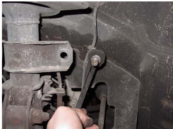
6. Remove stabilizer link from strut. ↑
