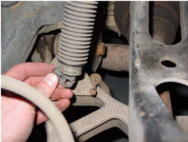
6. Unhook the height sensor arm. (Sensor is located on the driver side.) ↑
