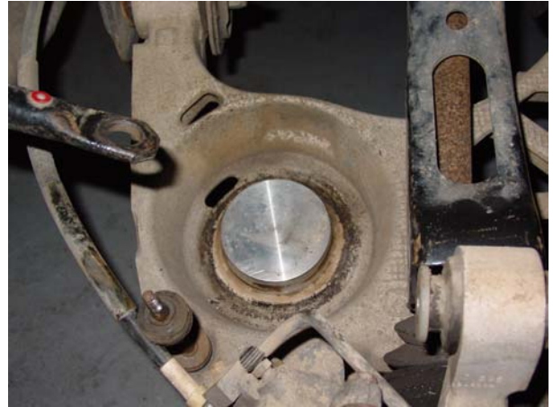
13. Install bottom spring seat in lower control arm. Bolt the aluminum spring pilot in place.
