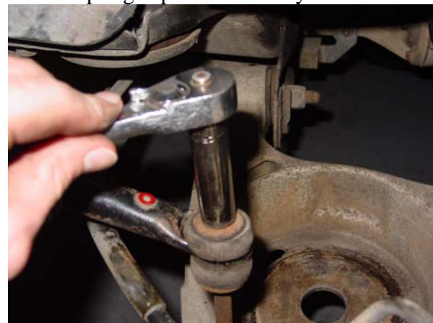
9. Disconnect the stabilizer bar link. ↑
