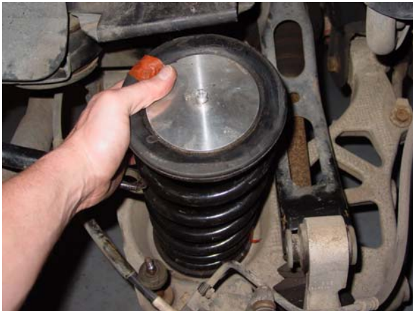
14. Carefully install the new rear coil spring over the bottom spring pilot. ↑
