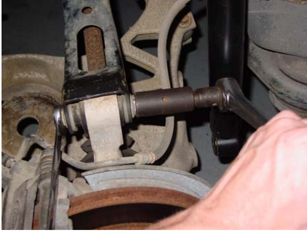
10. Remove upper rear suspension arm and bushing bolt and nuts.
