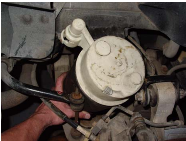
8. Remove air spring from lower control arm. ↑
