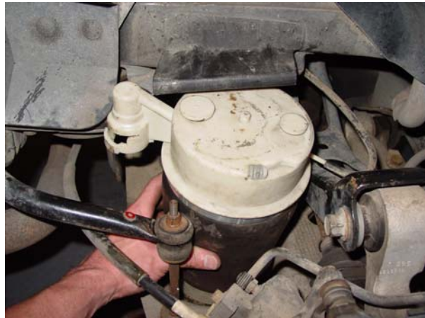
7. Hold down the metal locking tab at the top the air spring and rotate the spring to disengage the air spring cap from the body.
