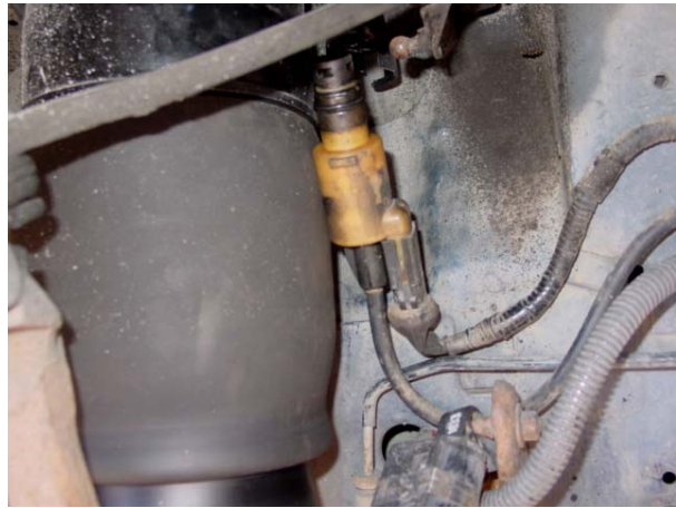
6. Rotate solenoid counterclockwise to the first stop, then pull down on solenoid. ↑ Rotate again and remove solenoid.
