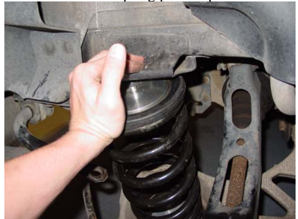
15. Spay the top of the coil spring with a lubricant. Push the top of the coil spring in place. Make sure the center Dow pin is in the correct hole.
