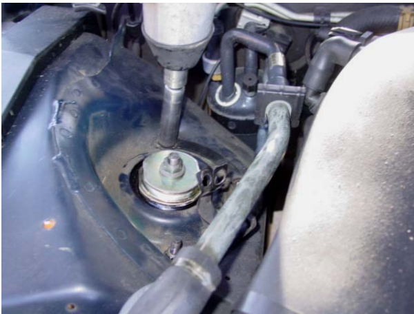
7. Remove the shock tower cover from over air spring attachments in engine compartment. Remove the three nuts retaining air spring.
