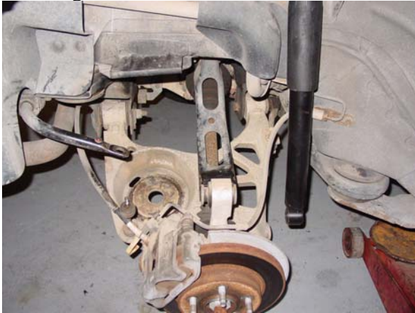
12. Rear suspension ready to install coil spring.
