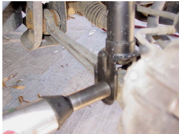
8. Remove lower nut and bolt to detach strut from front suspension arm support.
