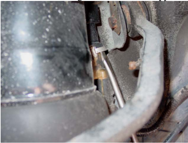
5. Remove solenoid-retaining clip. ↑
