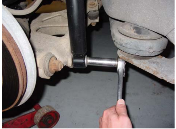
11. Remove bolt from the bottom of the rear shock.
