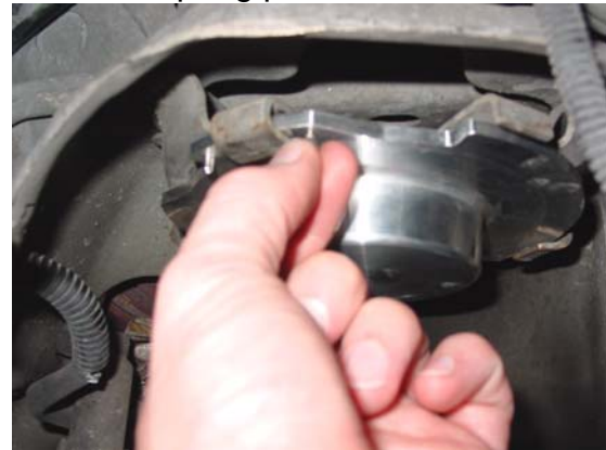
16. Replace setscrew in top plate, locking it from turning. ↑
