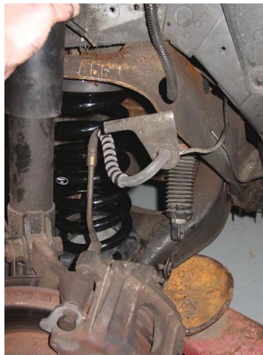
19. Compress the strut, and jack up on the lower control arm. ↑ MAKE SURE THE COIL SPRING IS LOCKED IN PLACE!!
