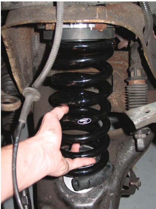
18. Install front coil spring. ↑ (Rotate spring so "Arnott Inc." logo faces the wheel.)
