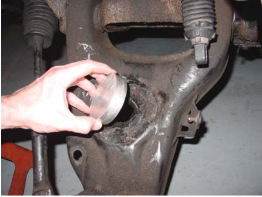
17. Bolt lower aluminum spring mount on to lower control arm. ↑
