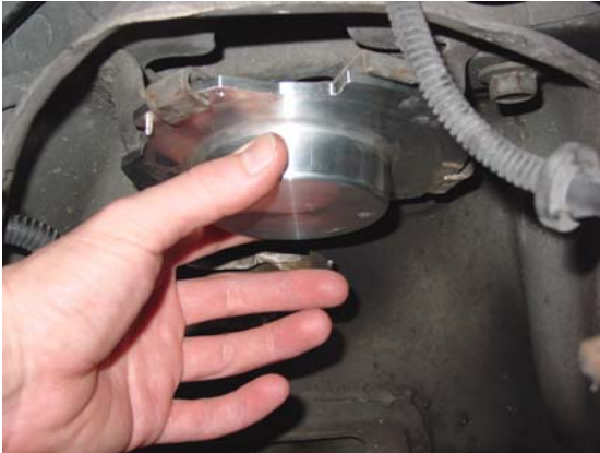
15. Rotate plate into top suspension bracket. ↑
