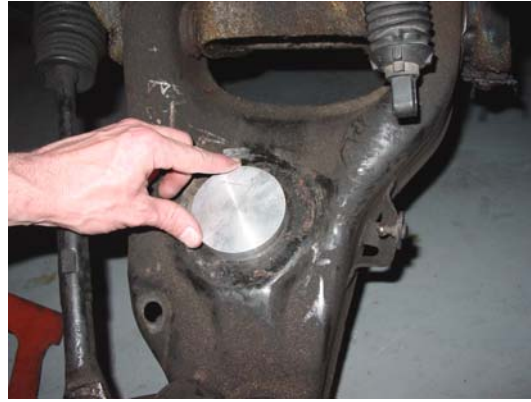
17. Bolt lower aluminum spring mount on to lower control arm. ↑
