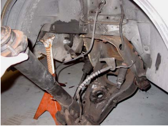
13. Push down on strut and pull towards you. (Do not pull on brake line!)
