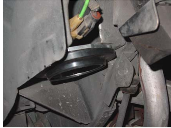
9. Install upper coil spring insulator. ↑
