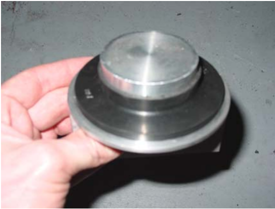
10. Install lower coil spring insulator on lower spring mount. Bolt the lower spring mount in the lower control arm. ↑
