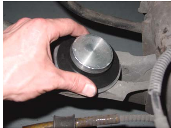
10. Install lower coil spring insulator on lower spring mount. Bolt the lower spring mount in the lower control arm. ↑
