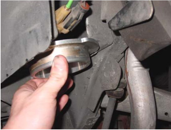
8. Install upper coil spring mount. ↑ After installing, replace setscrew.
