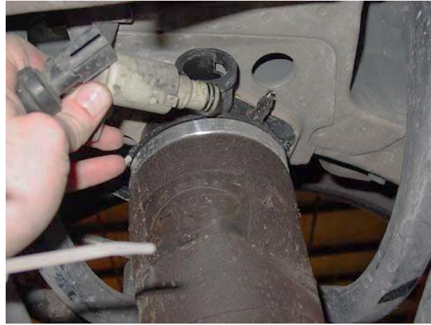
5. Rotate solenoid counterclockwise to the first stop, then pull outward on solenoid. Make sure all the air vents out of the air spring. ↑ Rotate again and remove solenoid.
