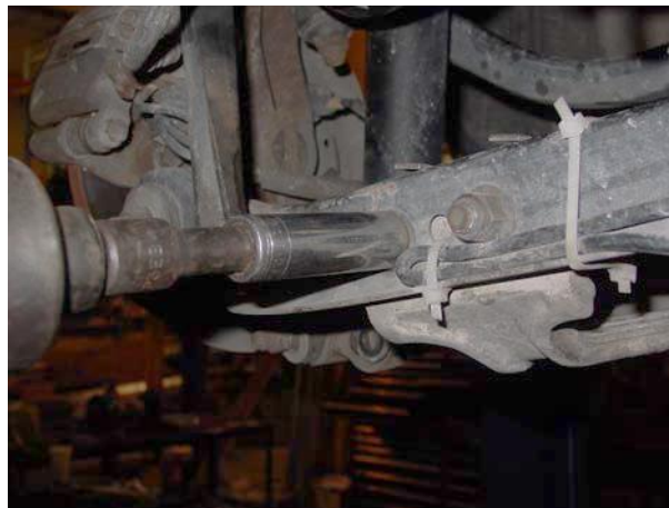
10. Remove lower spring seat nuts and bolts. ↑
