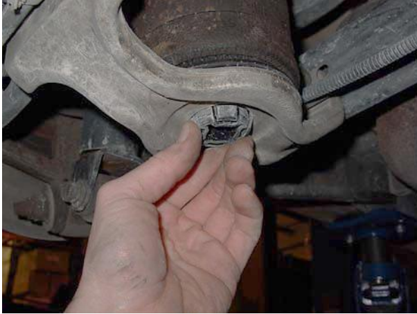
8. Depress the four locking clips on the lower air spring piston. Push up through spring seat. ↑
