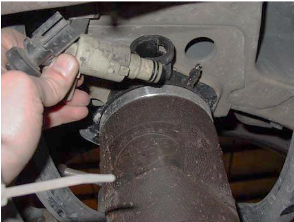
6. Remove air hose and unplug power to the solenoid. To remove the air hose, push down on the orange ring while pulling out on the nylon tubing. ↑
