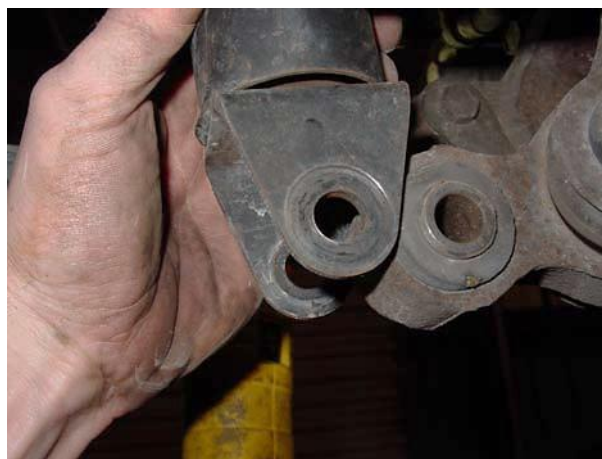
12. Unbolt the top and bottom shock absorber retaining nuts and bolts. ↑
