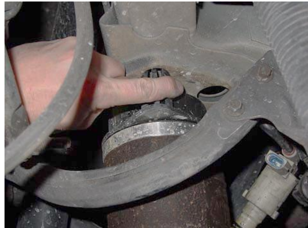
7. Depress the two plastic locking fingers on the top air spring cap. Push down on air spring and remove from top body bracket. ↑
