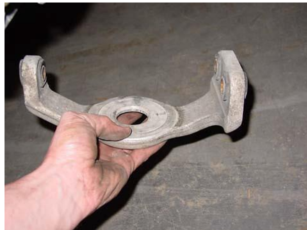
11. Remove lower spring seat. ↑
