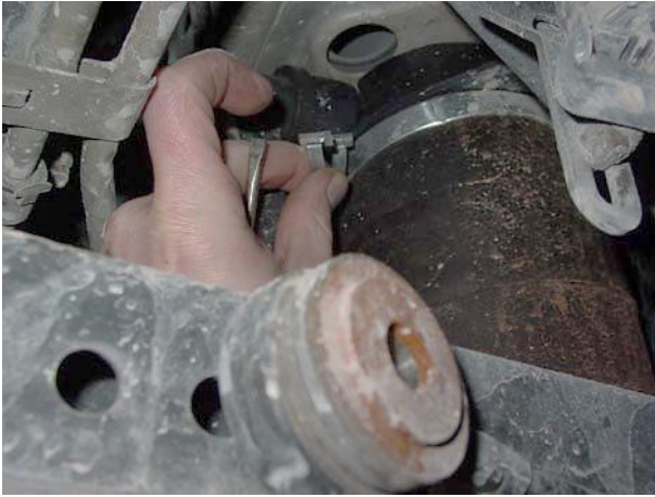
4. Remove solenoid-retaining clip. ↑
