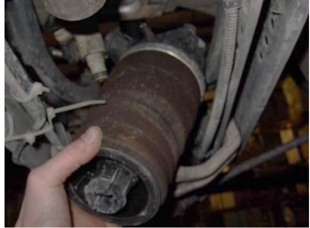
9. Remove old air spring from vehicle. ↑
