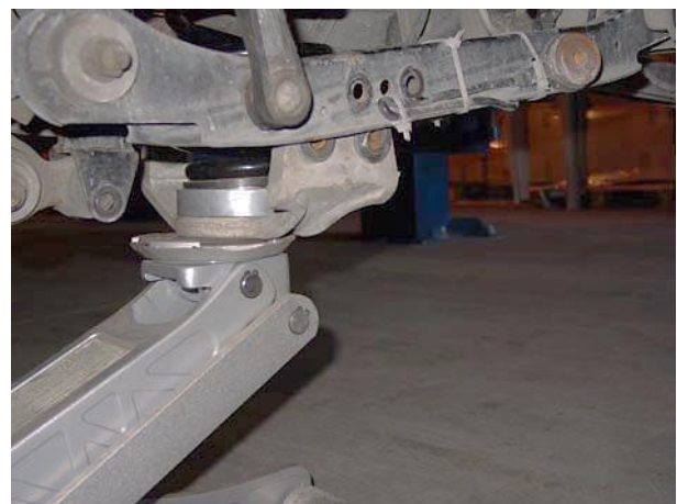
13. Install coil spring to upper and lower spring mounts using the aluminum spring mounts supplied with conversion kit. (Very carefully, jack up on the center of the lower spring seat). ↑
