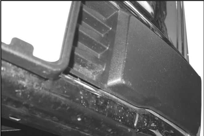
(Fig 4) Remove bumper pads to access splash guard hardware if necessary. 2017 F150 pictured
