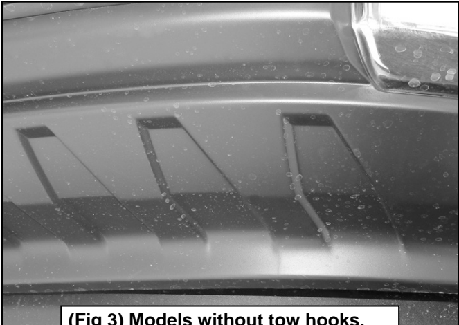
(Fig 3) Models without tow hooks, temporarily remove the plastic splash guard and spoiler if equipped
