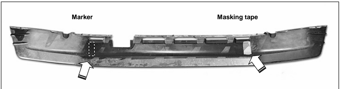
(Fig 16) Use removable tape (masking tape) or a marker to mark location of Frame Brackets onto back of air dam (arrows). Carefully cut small openings with a sharp knife or hacksaw blade. Guide marks pictured for example only. Check location and measurements of all guide markings before cutting.
