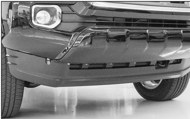
(Fig 1) Remove air dam from bottom of bumper
