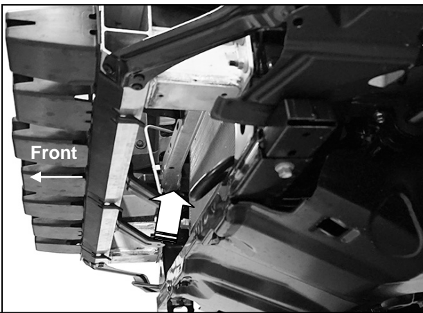
(Fig 8) Plastic bumper removed for instruction purposes only-do not remove bumper
