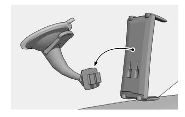
Insert device by pushing down on the lower support legs and engaging the spring-loaded mechanism. Adjust support legs as necessary.
