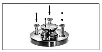
**3** Replace the mount over the base. Tighten knob to secure.
