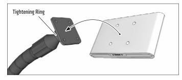
**Optional:** Attach included metal conduit to console to minimize vibration.
