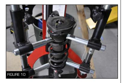
12. It is recommended to use proper spring compressors before removing the top nut on the strut tower using the 17 mm socket wrench then remove the OEM spring (Figure 10)
