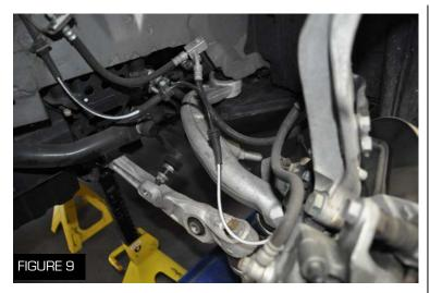
11. After removing the OEM shock and spring, be sure to remember where everything goes for the installation (Figure 9)
