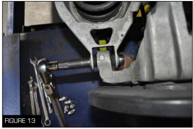
1. Remove the rear wheels using the proper 3. Unbolt the spring assembly using a 17 mm socket or key for the lug nuts or wheel locks socket wrench and 17 mm wrench (Figure 13) (Figure 11)
