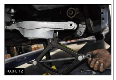
2. Put the scissor jack under the brake assembly to support it (Figure 12)
