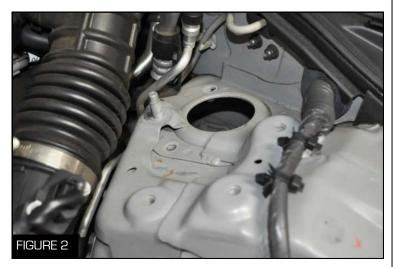
3. Remove the OEM strut bar using the 14 mm socket wrench (Figure 2)
