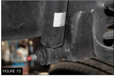
3. Unbolt the nut on the strut using a 19 mm socket wrench (Figure 11)
