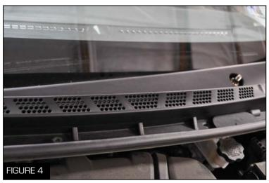
5. Remove the 4 plastic clips on the plastic cover using a flat head, you must push the center down first then pull up on the clips (Figure 4)
