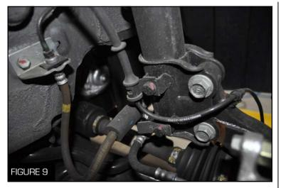
11. Unbolt the two smaller bolts for the brake line using a 12 mm socket wrench (Figure 9)
