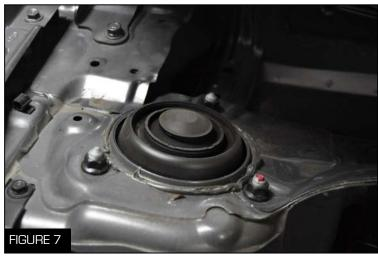
8. Unbolt the top 3 nuts on the strut using a 14 mm socket wrench (Figure 7)
