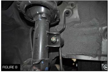
10. Unbolt the sway bar end link with a 19 mm socket wrench (Figure 8)
