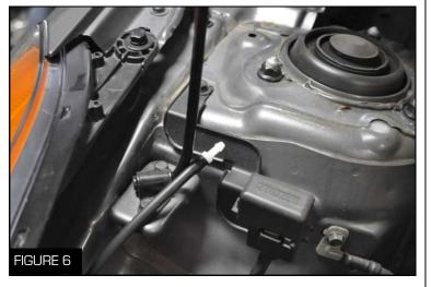
7. Unplug the windshield wiper washer fluid hose from the plastic cover (Figure 6)
