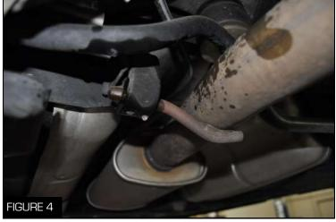
4. Spray the metal hanger and rubber insulator on the resonator pipe (Figure 4)
