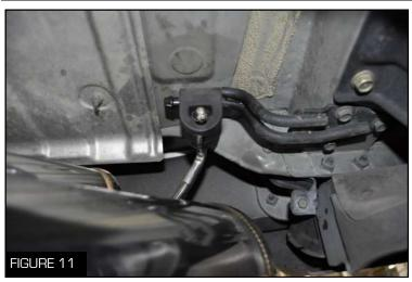
7. Spray the two metal hangers and rubber insulators with a lubricant and slide the hangers into the insulators for both mufflers (Figure 11)
