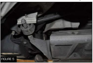
6. Spray the metal hanger and rubber insulator on the side of the muffler facing the front of the vehicle with a lubricant (Figure 5)
