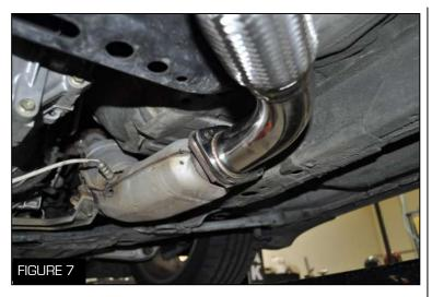
1. Bolt the X-pipe to the OEM catalytic converters with the OEM gaskets, nuts, and bolts using a 14 mm socket wrench (Figure 7)
