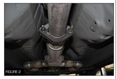
2. Unbolt the Y-pipe from the resonator pipe section using a 14 mm socket wrench and remove the Y-pipe from the vehicle (Figure 2)
