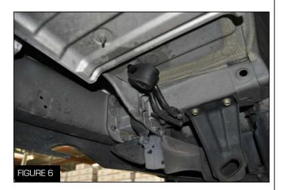
7. Spray both metal hangers and rubber insulators on the rear-facing side of the muffler and then remove the muffler from the vehicle (Figure 6)
