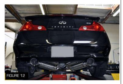
8. Have one person align the mufflers and tips while the other person tightens down all of the nuts and bolts to the proper torque specs (Figure 12)
