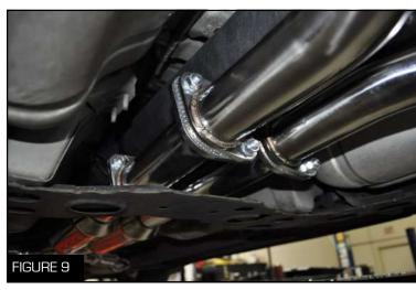
4. Bolt the mid pipes to the X-pipe with the supplied gaskets, nuts, and bolts using both 16 and 17 mm socket wrenches (Figure 9)
