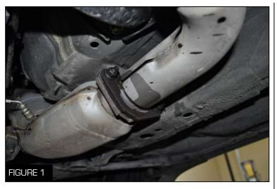
1. Unbolt the Y-pipe from the catalytic converters using a 14 mm socket wrench (Figure 1)
