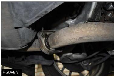
3. Unbolt the resonator pipe from the muffler using a 14 mm socket wrench, move the grounding wire out of the way (Figure 3)
