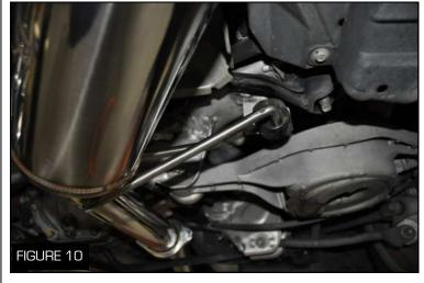
5. Spray the metal hanger and rubber insulator for the muffler with a lubricant (Figure 10)
