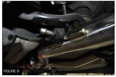
2. Spray the metal hanger and rubber insulator for the mid pipe with a lubricant (Figure 8)
