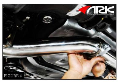
sliding the metal hanger from the mid pipe into it (Figure 4)
