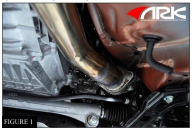
1. Optional part: Bolt the resonated test pipe to the OEM catalytic converter with the OEM flange gasket and nuts using a 17 mm socket wrench (Figure 1)
