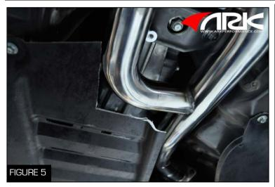
8. To put the shield back on with the ARK Performance test pipe, you must cut out the corner to clear the resonator (Figure 5)
