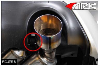
9. Spray the rubber insulators for the muffler and slide the metal hangers into them (Figure 6)
