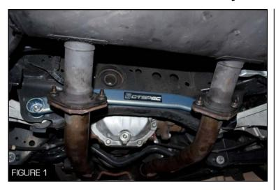
1. Unbolt the muffler from the mid pipe using a 14 mm socket wrench (Figure 1)
