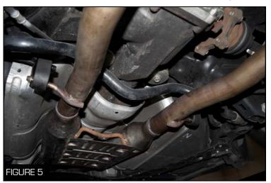
5. Spray the rubber insulators and metal hangers with a lubricant on either side of the mid pipe and slide the hanger out of the insulators (Figure 5)
