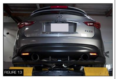
6. It is recommended to have someone help align the tips and mufflers while someone else tighten down all of the nuts and bolts to the proper torque specs (Figure 13)
