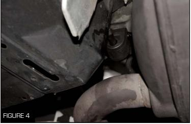
4. Spray the rubber insulator and metal hanger on the passenger side of the muffler with a lubricant then slide the hangers out of the insulators and remove the muffler from the vehicle (Figure 4)
