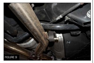
2. Spray the rubber insulator and metal hangers on both sides of the X-pipe with a lubricant and slide the hangers into the insulators (Figure 9)
