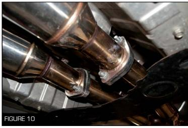
3. Bolt the X-pipe to the front resonator pipes with the supplied nuts, bolts, and gaskets using a 16 and 17 mm socket wrench (Figure 10)
