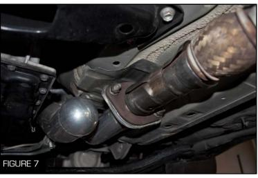
7. Unbolt the Y-pipe from the catalytic converter (aftermarket test pipe shown) using a 14 mm socket wrench and remove the Y-pipe from the vehicle (Figure 7)
