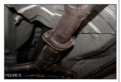
6. Unbolt the mid pipe from the Y-pipe using a 14 mm socket wrench and remove the mid pipe from the vehicle (Figure 6)
