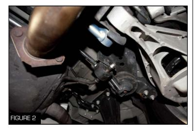
2. Spray the rubber insulator and metal hanger on the muffler with a lubricant (Figure 2)
