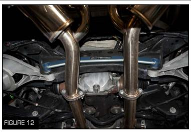
5. Bolt the mufflers and the X-pipe with the supplied bolts, nuts, and gaskets using both 16 and 17 mm socket wrenches (Figure 12)
