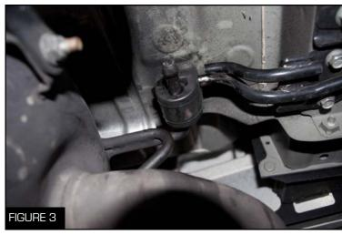
3. Spray the rubber insulator and metal hanger on the driver side of the muffler with a lubricant (Figure 3)
