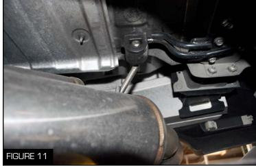
4. Spray both rubber insulators and metal hangers for the mufflers with a lubricant and slide the hanger into the insulator (Figure 11)
