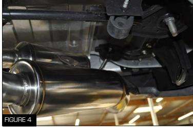
4. Spray the metal hangers and rubber insulators on the mufflers with a lubricant and slide the metal hangers into the rubber insulators towards the back of the vehicle (Figure 4)
