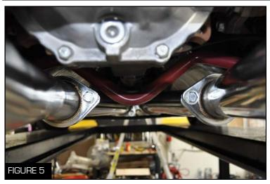
5. Bolt the mufflers to the mid pipes with the supplied gaskets, bolts, and nuts using both 16 and 17 mm socket wrenches (Figure 5)
