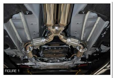
1. Bolt the X-pipe to the OEM catalytic converters using the OEM gasket and nuts (Figure 1)
