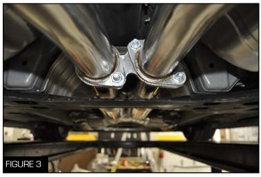
3. Bolt the mid pipes to the X-pipe with the supplied gaskets, nuts, and bolts using both 16 and 17 mm socket wrenches (Figure 3)
