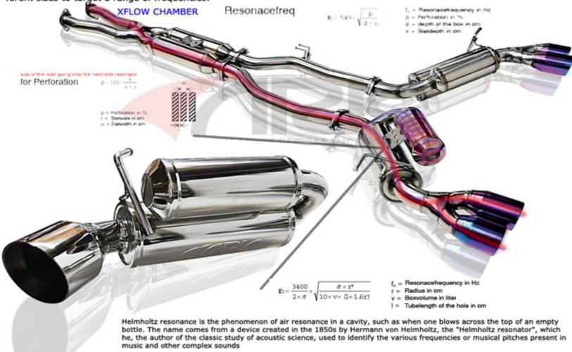
When air is forced into a cavity, the pressure inside increases. When the external force pushing the air into the cavity is removed, the higher-pressure air inside will flow out. However, this surge of air flowing out will tend to over-compensate, due to the inertia of the air in the neck, and the cavity will be left at a pressure slightly lower than the outside, causing air to be drawn back in. This process repeats with the
