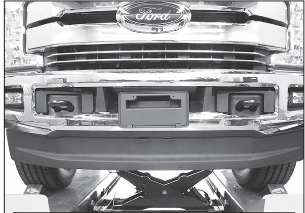
(Fig 6) Remove plastic air dam from bumper
