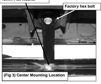
10mm-1.50mm x 45mm Hex Bolt Hex Bolt 10mm Lock Washer 10mm Flat Washer Actual brackets may have two holes here
