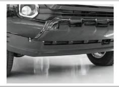
Locate and remove the factory hex bolt on the passenger side of the vehicle.
