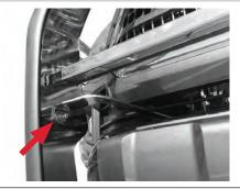
Once the grille guard is aligned, tighten all hardware.
