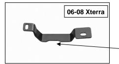
Driver/Left Side Short Top Bracket Pictured 05-08 Xterra Note position of notch for grille clearance
