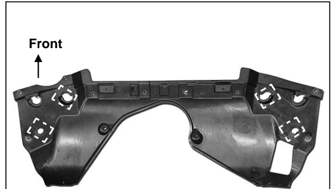
(Fig 19) Hold splash guard up to bottom of Brackets to determine areas to cut from cover. (Bottom of splash guard pictured)
