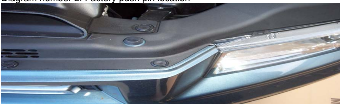
Diagram number 3. well nut installed under upper trim panel for braces bracket
