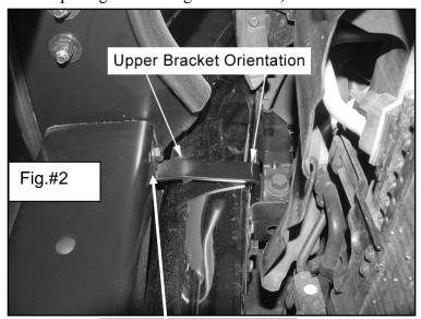
1pc M10 x 1" Hex Bolts 2pcs 10mm Oversized Flat Washer 1pc 10mm Lock Washer 1pc M10 Hex Nuts
