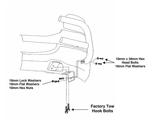
Figure 2 (Driver Side Installation Shown - Without Tow Hooks)
