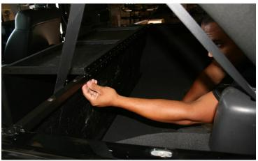
STEP 6: TAKE THE 8MM X 40 BUTTON HEAD BOLT AND ATTACH THE 8MM NUT (THIS WILL ACT AS A LOCK DEVICE). MOUNT THE 8MM BUTTON HEAD AND NUT TO THE BACK BOTTOM END OF THE PASSENGER SIDE CARGO PLATE. SCREW IN ALL THE WAY TO BOTTOM, YET NOT TIGHT. THE CARGO PASSENGER PLATE NEEDS TO BE FITTED TO VEHICLE, AND THEN ADJUSTMENT MADE TO THE 8MM BOLT SO THAT IT STABILIZES THE CARGO PLATE (ADDING ADDITIONAL SUPPORT).
