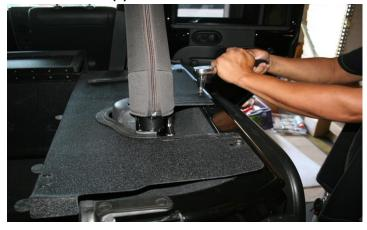
\*JEEP JK HARDTOPS WILL NOT REQUIRE (3) 8MM X 35 BOLTS, (3) 8MM NUT PLATES, NOR WASHERS.. USE EXISTING HARDWARE
