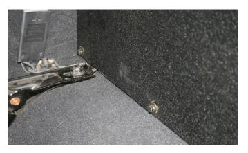
**STEP 4:** WITH THE HELP OF ANOTHER PERSON ALIGN THE CARGO CENTER PLATE & LID ON TOP OF THE BACK SEAT PLATE. UNFOLD THE CARGO CENTER PLATE (FACING TOWARDS THE REAR OF VEHICLE) TO SIT AT A 90 DEGREE ANGLE. THIS WILL STABILIZE THE CARGO CENTER PLATE.
