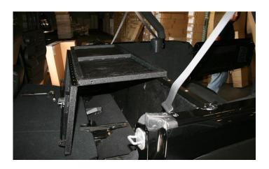
**STEP 5:** ONCE STABLE, MOUNT THE CARGO CENTER PLATE TO THE BACK SEAT PLATE USING (10) 8MM X 35MM BOLTS WITH 8MM LOCK AND FLAT WASHERS. LEAVE SEMI LOOSE FOR ADJUSTMENT.
