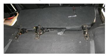
**STEP 3:** ALIGN THE CARGO BACK SEAT PLATE TO THE EXISTING OUTER HOLES. THE CARGO BACK SEAT PLATE WILL BE UPRIGHT. INSTALL USING THE EXISTING OUTER BOLTS. TIGHTEN IN PLACE SECURELY.
