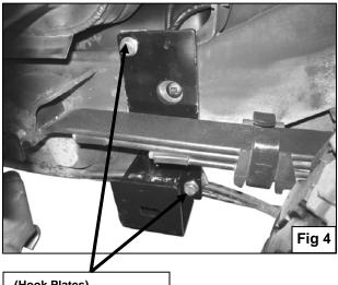
(Hook Plates) 12mm x 45mm Hex Bolts 12mm Lock Washers **12mm Flat Washers**
