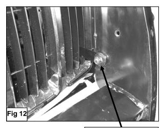
10mm x 30mm Button Bolt 10mm Lock Washer 10mm Hex Nut 10mm Flat Washers
