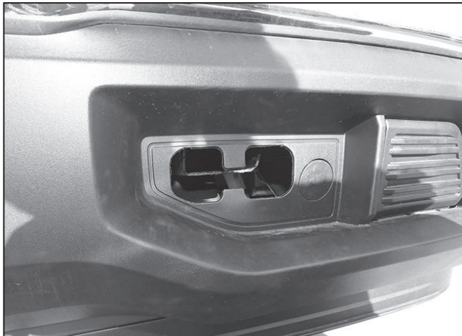
(Fig 3) Tow hook removed. Opening may need to be trimmed to clear the Mounting Bracket assembly
