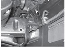
On the 2014 - 15 models, from behind the bumper, remove the clips securing the fascia to the top of the bumper.
