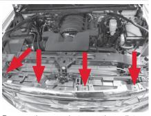
Remove the cover between the radiator and the grille. Remove the screws attaching the top of the grille (arrows).
