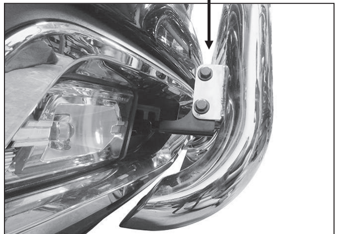
(Fig 13) Passenger/right side complete installation
