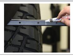
Using a square, draw a cut line around the hanger to help create a straighter cut.
