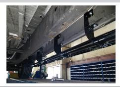
Carefully place the side bar on the brackets with the larger step pad toward the front of the vehicle.
