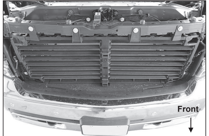
(Fig 13) Remove screws attaching grille and carefully pull grille straight out to remove grille
