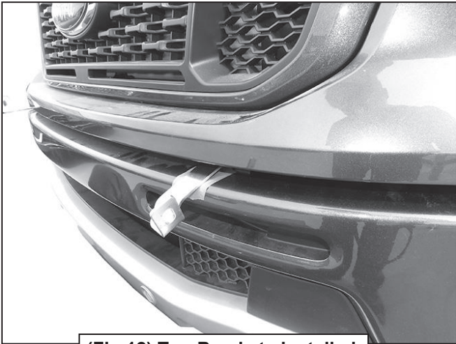
(Fig 12) Top Brackets installed
