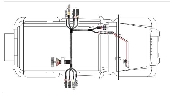
On the driver side, take the power wire and sensor wire (orange / yellow) and route it to the front of the vehicle underneath the carpet.
