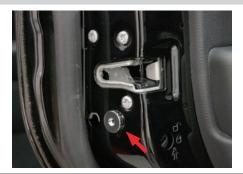
On the driver side, plug the rear actuator (red / black) into the running board and pull the extra wire back into the vehicle.
