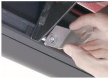
At this time, adjust the running board to the desired location.
