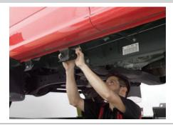
With the driver-side brackets installed, take the driver-side running board and insert three T-rails into the slot as shown.
