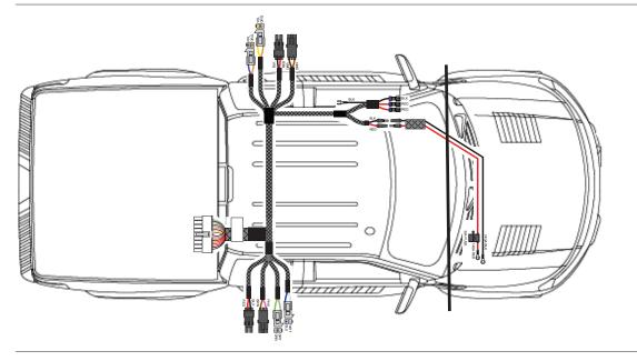
On the driver side, take the power wire and sensor wire (orange / yellow) and route it to the front of the vehicle underneath the carpet.
