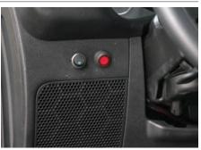
Locate a suitable location to connect the ground wire for the LED on the switch behind the dash panel.
