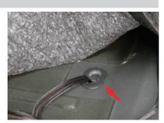
If there is no plug in the floor behind the driver seat, locate a position close to the rear bracket and drill a 1" hole through the floor of the vehicle.
