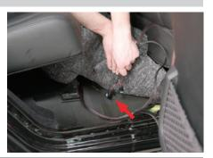
Plug the door sensor into the wiring harness and route it up the door frame, under the carpet.
