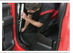
Once the trim panels are removed, take the second section of wiring harness and route it under the carpet, through the vehicle, from the passenger-side rear to the desired location.
