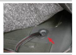
Plug the door sensor into the wiring harness and route it up the door frame, under the carpet.
