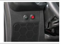
Locate a suitable location to connect the ground wire for the LED on the switch behind the dash panel.
