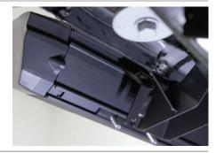
Secure the running board to the front mounting bracket using one M8 flat washer and one 5/16" nylock nut on each T-rail stud.
