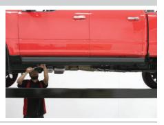
On the front passenger-side mounting location, locate the threaded hole on the inside of the body panel and place an L-bracket on to that panel.
