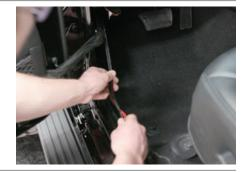
Remove the fasteners securing the front and rear door trim panels on both sides of the vehicle. There are five clips on each side of the vehicle securing the trim panels, three for the front and two for the rear.
