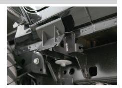
With the passenger-side brackets installed, take the passenger-side running board and insert three T-rails into the slot as shown.
