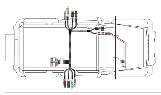
On the driver side, take the power wire and sensor wire (orange / yellow) and route it to the front of the vehicle underneath the carpet.
