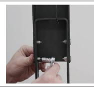
Lay the factory spare tire carrier on a flat surface and remove the four T-25 torx screws securing the light to the housing.
