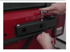
Repeat step 6 to remove the lower factory door hinge. Loosely install the lower HD replacement hinge following step 7.
