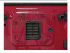
Moving on to the hinge location, remove the plastic covers to expose the factory hinge mounting hardware.
