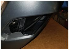
With the light removed, detach the side marker light.
