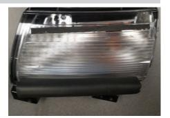
Once the seal is in place, install the light into the bumper corner using an M4 button head bolt, lock washer and flat washer.
