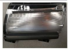
Once the seal is in place, install the light into the bumper corner using an M4 button head bolt, lock washer and flat washer.
