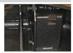
Take C-channel bracket and place it into the frame of the Jeep.
