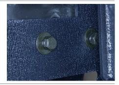
Secure the corner bumper bracket to the vehicle with M10 hex bolts, lock washers and M10 x 27mm flat washers.
