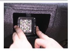
Once the LED lights and switch are installed, connect the harness extension to each light. Insert the male plug on the harness extension into the female socket on each LED light.
